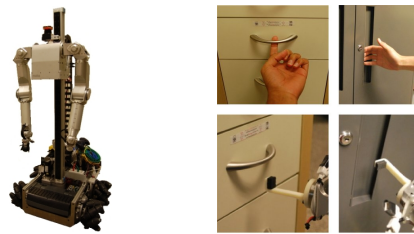
Fig. 2. Left: The mobile manipulator used in this work. Right: Examples of a human using his hand as a hook and corresponding orientations for the robot’s hook end effector.
