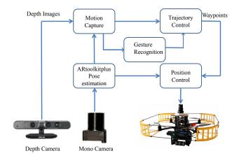
Fig. 3. System overview. We use a depth camera on a flying platform to detect a person. We stabilize the depth image based on the current pose estimate of the quadrocopter.
