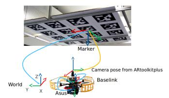
Fig. 5. Static transformations are shown in blue whereas camera pose is estimated in realtime and is shown in yellow
