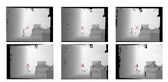
Fig. 7. Visualization of the raw and the stabilized depth images with camera motion along a square trajectory (top and bottom row respectively). The red dot always marks the same (absolute) pixel in the image. As can be seen, the red pixel jumps significantly in the raw images, while it remains stable in the stabilized ones.
