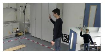
Fig. 1. Our approach enables a quadrocopter to follow a person and to understand simple gesture commands such as "follow me", "take picture", and "land".
