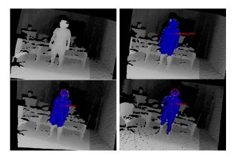
Fig. 8. Illustration of robust person tracking with stabilized depth video. The OpenNI tracker successfully initializes tracking, although the real depth camera undergoes a strong motion.
